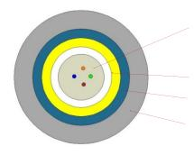
• **Uni-tube:** thermoplastic material, containing up to 24 fibres and filled with a suitable water tightness compound.
